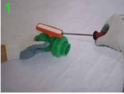
1 Sap kapağı yerinden çıkarılır Lid of handle is removed from its place
