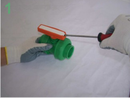
Sap kapağı yerinden çıkarılır Lid of handle is removed from its place
